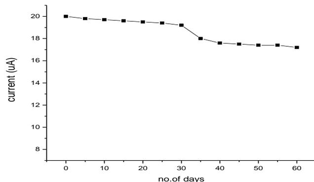
**Fig. 7.** Stability of the Gr/POA/Ache electrode storage for 60 days.
