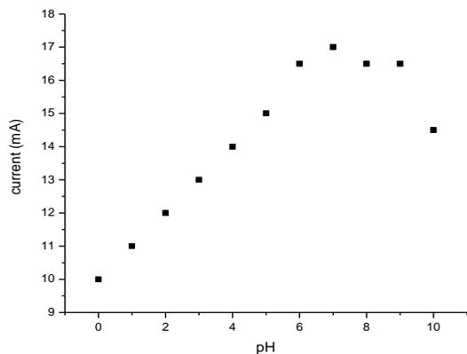
**Fig. 5 (a).** Effect of pH on Gr/POA/AChE at potential 0.5V.
