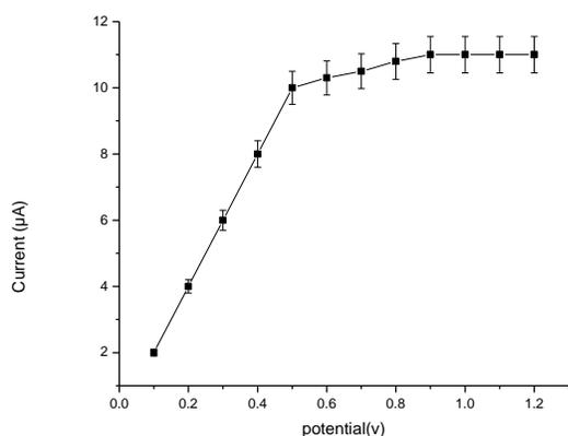
**Fig. 4.** Effect of potential on Gr/PANI/PNP electrode.
