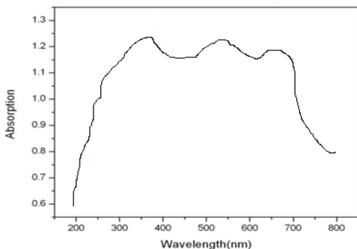
**Fig. 2.** UV-visible spectrum of sensor Gr/POA/AChE.
