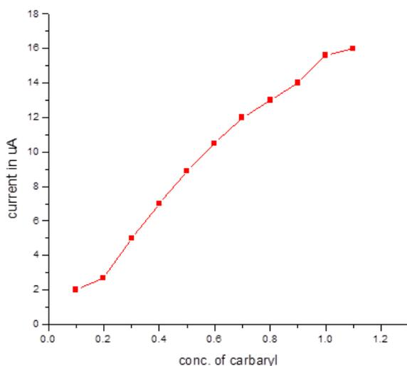
**Fig. 6.** Amperometric response of Gr/POA/Ache.
