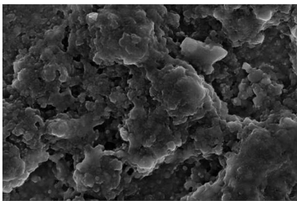
**Fig. 3.** SEM image of Gr/POA/AChE at 20µM.
